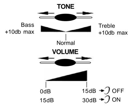
Note: When the tone (treble), earpiece volume and sending levels are set to the maximum, whistling may appear. If whistling occurs the sending level settings should be decreased (sending level switch located on the right side). When the switch located behind the phone is **ON**, the extra-receiving and tone functions are automatically activated each time you use the phone. When the switch switch of switched **OFF**, you will need to activate the function by pressing the button .
